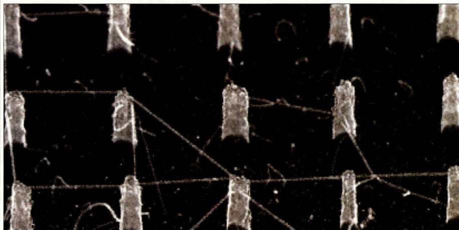
Nanotube networks – this scanning electron microscope picture shows carbon nanotubes draped across silicon pillars. The spacing between pillars is 500 nm.
