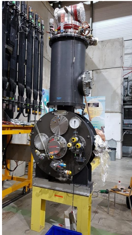
Fig. 1.5 – Central cryostat and its vacuum enclosure of COMPASS target.
