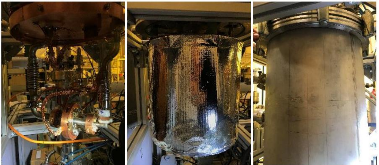
Fig. 4.2 – Pictures of the inside of the cryostat, showing: Left) thermalized sample (Cu ring), middle) thermal shield with Multi-Layer Insulation (MLI) cover, right) closed vacuum vessel.
