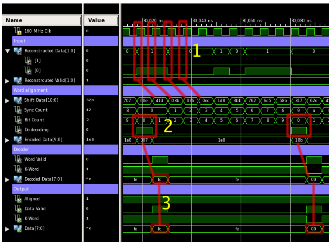
Figure 7.23: Simulation of the Word Alignment and 8b10b decoder block.
