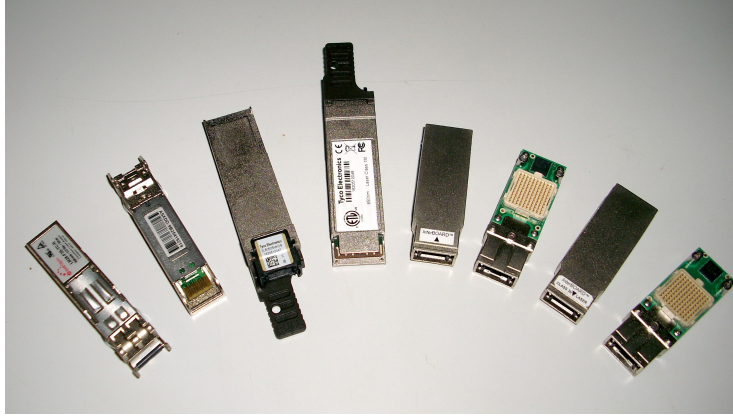
Figure 7.3: 3 types of industrial optical modules, each shown from the electrical connector and the optical connector side. From left to right: SFP, QSFP, Snap12 TX, Snap12 RX.
