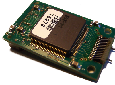
Figure 5.7: Picture of a TX plugin used on the BOC to BPM encode the TTC signal and convert them into optical signals.
