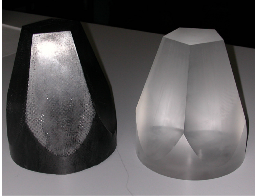
Figure 4.6: Single crystal of the Total Absorber Calorimeter at n_TOF and respective carbon capsule
