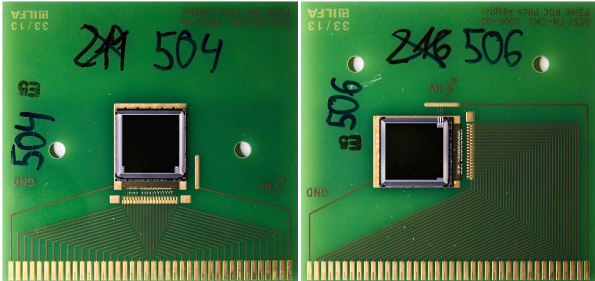
Figure A.4: CMS SCM assemblies for the test beam measurements. Due to mechanical constraints, one of the samples is mounted upright, the other one rotated by 90^\circ to allow for tilting of the sensor plane in both column and row direction.
