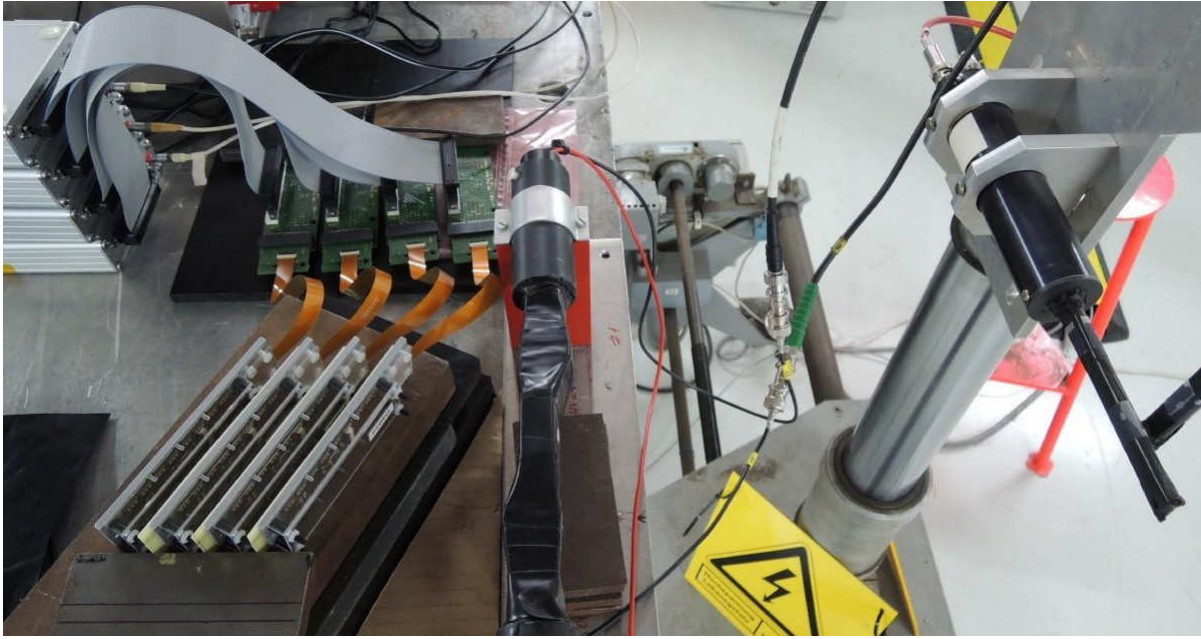
Figure D.3: Four CMS Pixel Detector modules operated in parallel. The modules are read out separately by four DTBs (top left) and triggered by two scintillators in coincidence (right). The planes are inclined for charge sharing. From [265].
