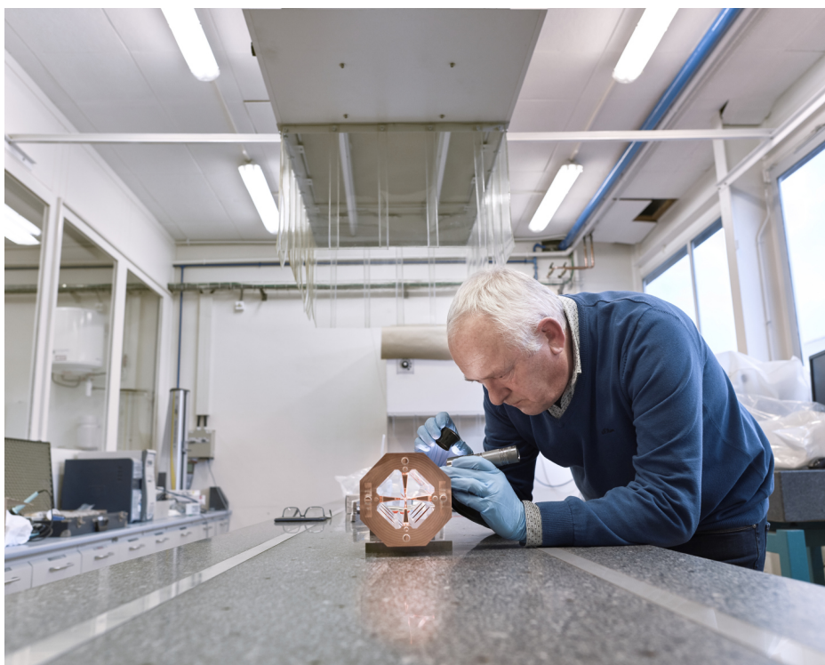
The radio-frequency quadrupole of the MACHINA project under development (Image: Julien Marius Ordan/CERN)
