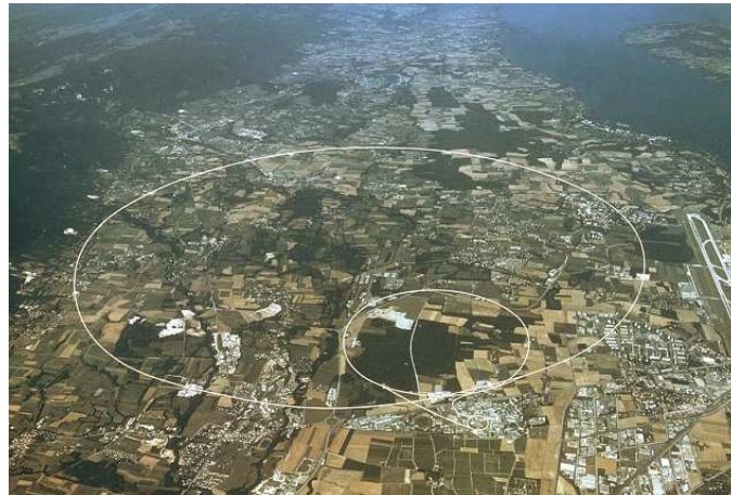
Figure 2.1: Aerial view of CERN and the surrounding region. The three drawn rings show the position of the accelerator complex located underground. The small ring is the Proton Synchrotron (PS), the middle ring is the Super Proton Synchrotron (SPS) and the largest ring is the Large Hadron Collider (LHC) [CERN1991].
