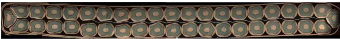
Figure 3.6: Cross-section of keystoneed 40-strand (0.7 mm diameter) Nb 3 Sn Rutherford cable with an 11 mm wide and 25 \mu m thick stainless-steel core [Fer2017].
