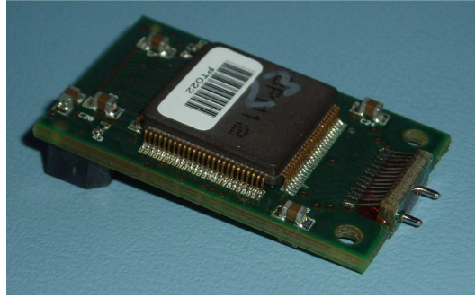
Figure 4.5: TX-plugin for transmitting the light from the BOC card to the opto-board. The size is 1.5 \times 3.5 \text{ cm}^2 .
