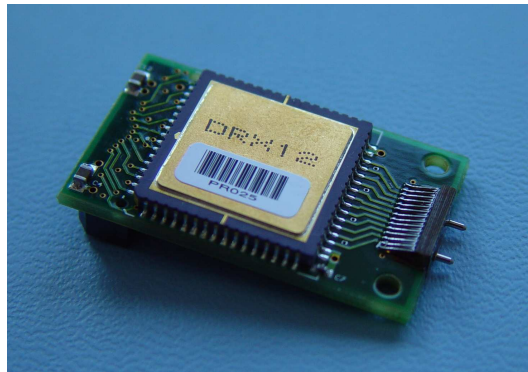
Figure 4.7: The RX-plugin is the optical to electrical converter housed on the BOC card. The size is 1.5 \times 3.5 \text{ cm}^2 .
