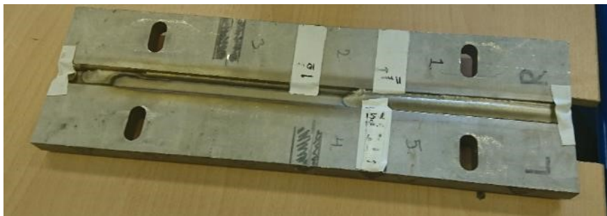
Figure B.9: Flat sample with artificial defects machined in five different "weld areas".
