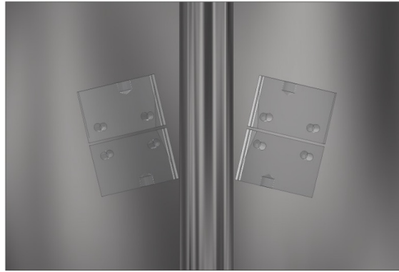
Figure 5.23: Top view illustration of one of the 15^\circ skewed probe scans. The scanning direction is along the weld, i.e. up or down of the paper.
