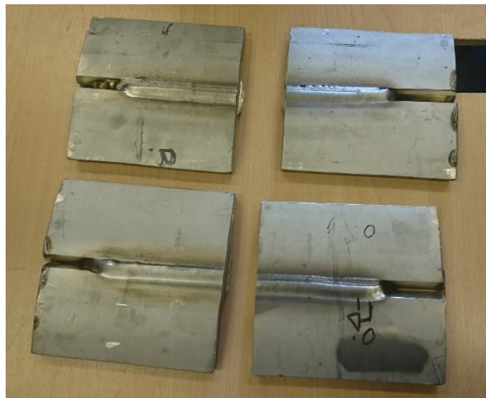
Figure B.11: 4 weld samples from an 11 T single aperture short model without any artificial defects.
