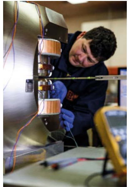
Magnetic Field Measurements on a Dipole Magnet.
