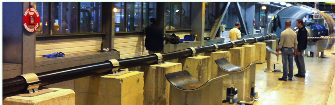
Figure 2: the black tube is the semi-flexible cryostat that will cool the \text{MgB}_2 cables from the tunnel to the surface. This particular tube, which is currently in SM18 undergoing testing, is 20 metres long with a diameter of approximately 16 cm.
