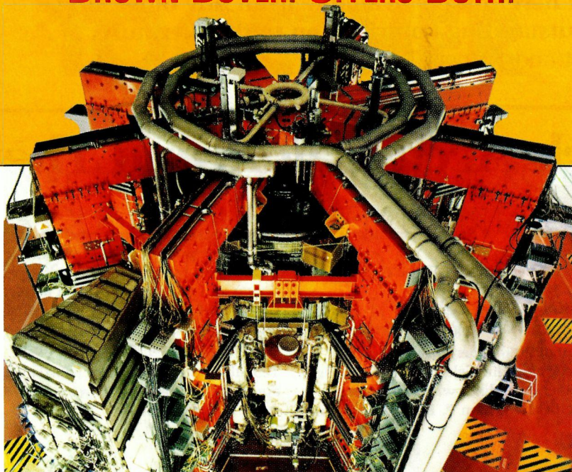
General view of JET, Joint European Torus at Culham, Oxfordshire, GB. For this test tokamak for plasma research BBC has delivered all toroidal field coils, the inner poloidal field coils, the four larger outer poloidal field coils as well as the magnet core. (Photo JET).
