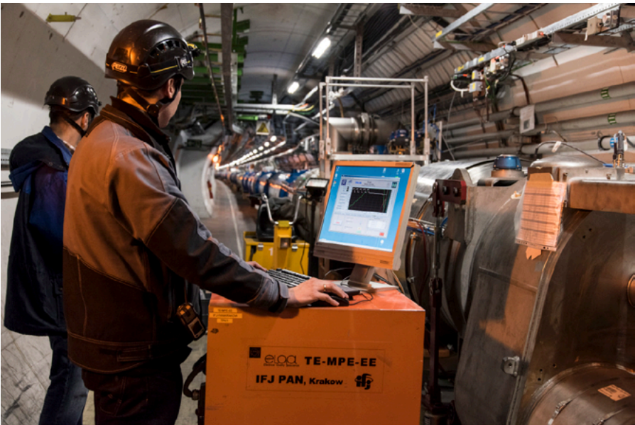
On Wednesday, 11 February at point 4 (sector 3-4), the teams in charge of the ELQA tests performed the final high-voltage qualification of an LHC main dipole insulation as part of an extensive series of LS1 interventions and upgrades. They applied 1500 V to the circuit and observed no significant leakage of current, which concludes the scheduled campaign of electrical tests positively.
