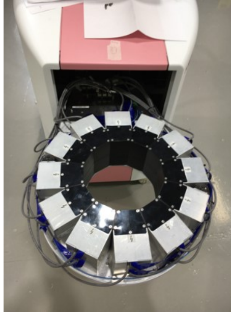
Figure 5.3: The PET ring in the MAMMI PET, without its plastic casing, consisting of two ring on top of each other, each with 12 scintillating crystals.
