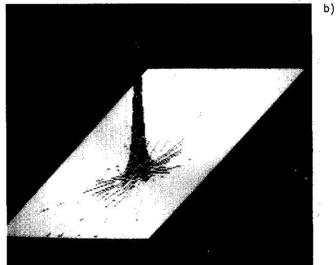
Fig. 6 Transverse section through a point source: a) back-projection; b) reconstruction.
