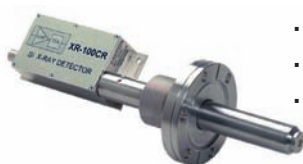
XR100CR fitted for vacuum applications
