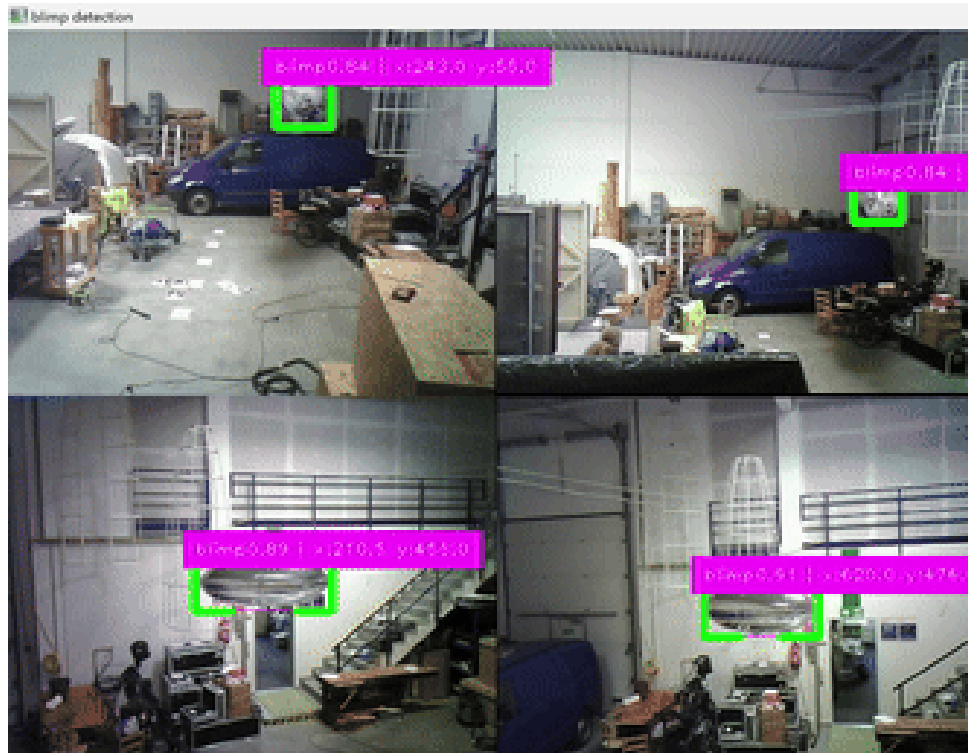
Figure 18: Example prediction result of model “20240807-py”: recognised blimp with different angles in same video input.
