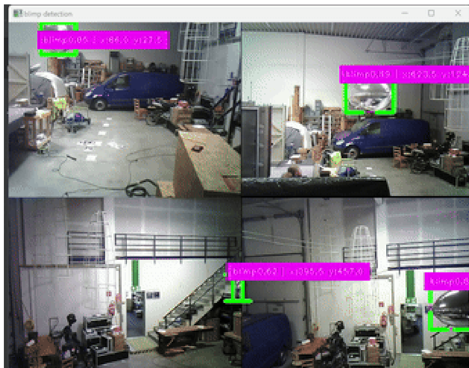
Figure 19: Example prediction result of model “20240808-py”: partial-displayed blimps are also recognized.
