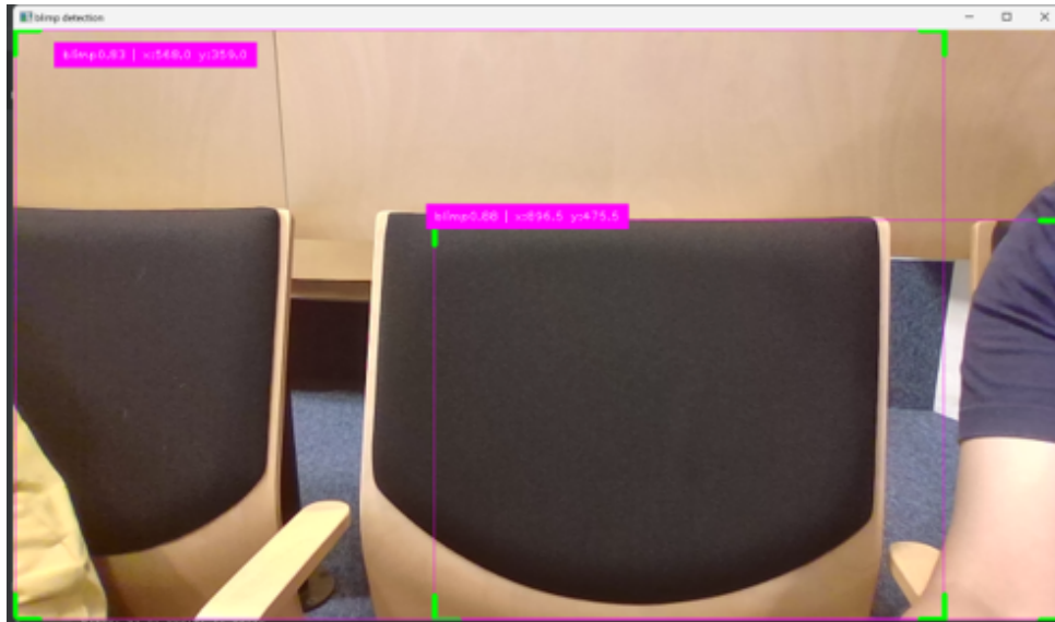
Figure 13: Example prediction result of model “20240731-py”: Chair and wall detected as a blimp.
