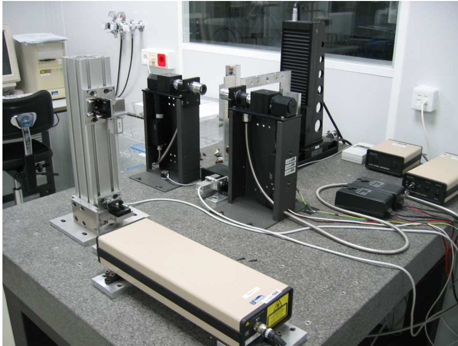
Figure 3.22: Photograph of the metrology setup used to survey the SCT end-cap modules assembled at IFIC (Valencia).
