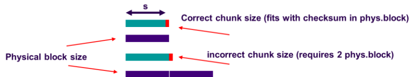
Figure 10: ensuring that the checksum information fits in the block size
