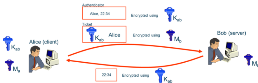
Figure 21: Example of a (simplified) mutual Kerberos authentication
