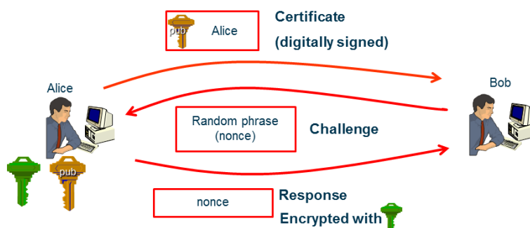
Figure 19: Authentication with certificate (simplified)
