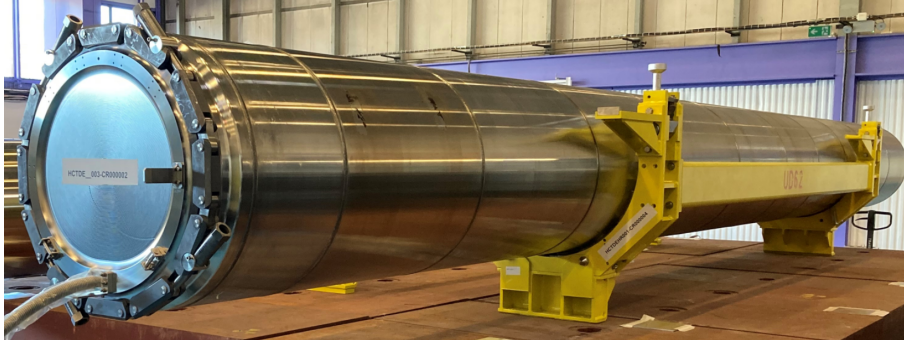
Figure 2.7: Run 3 dump block installed in its new support system.
