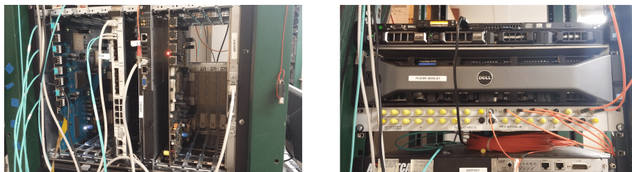
Figure 5.5: Left: two ABBAs in the ATCA crate, one connected to the optical fibers (leftmost board in the crate) and one disconnected (rightmost board in the crate). Right: machines used for monitoring and reconfiguration.
