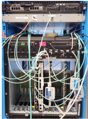
Figure 5.10: ATCA crate where three ABBAs and two machines are installed.
