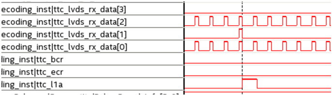
Figure 6.21: L1A detection and decoding in the TTC top level. The four LVDS lines (lvds_rx_data) with the synchronization pattern on the LVDS line 0, the channel B idle on the LVDS line 2 and the L1A on the LVDS line 2 are visible.
