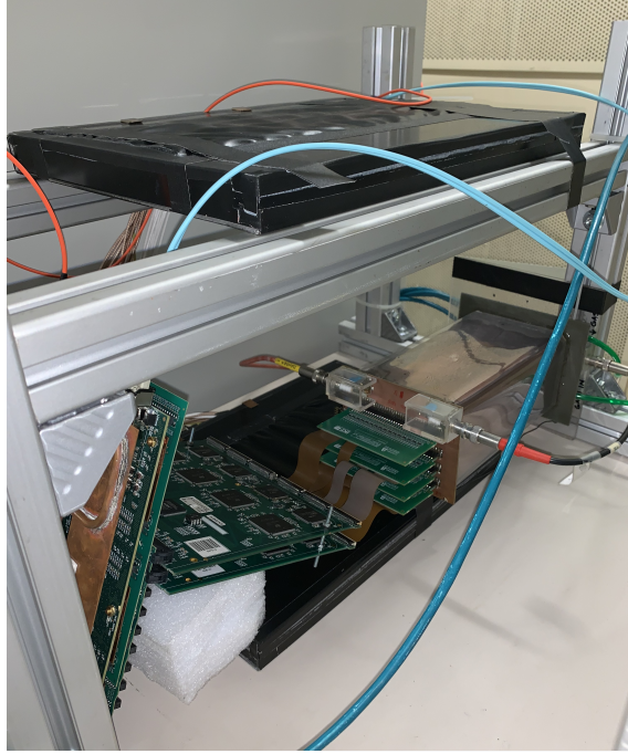
Figure 3: LMPD set-up: scintillators and PMTs on top and bottom, LMPD and front-end cards in middle.
