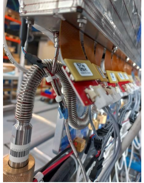
(b) Positioning of the CPS Dry Gas Outlet temperature sensor on the dry gas wire next to heating wires.
