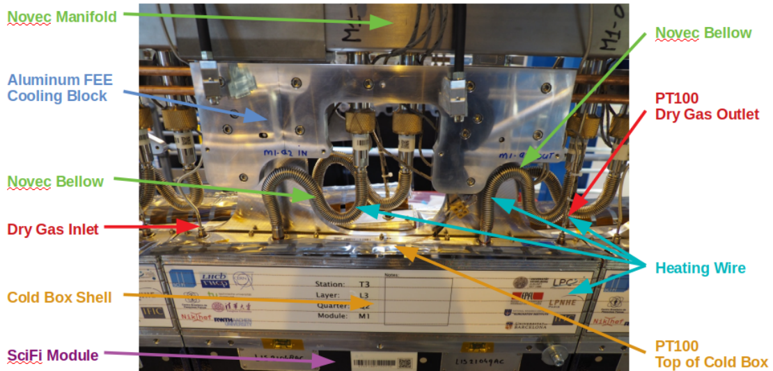
Figure 3: Location of temperature sensors and heating wires on the modules to prevent condensation in the detector. Taken from [2].
