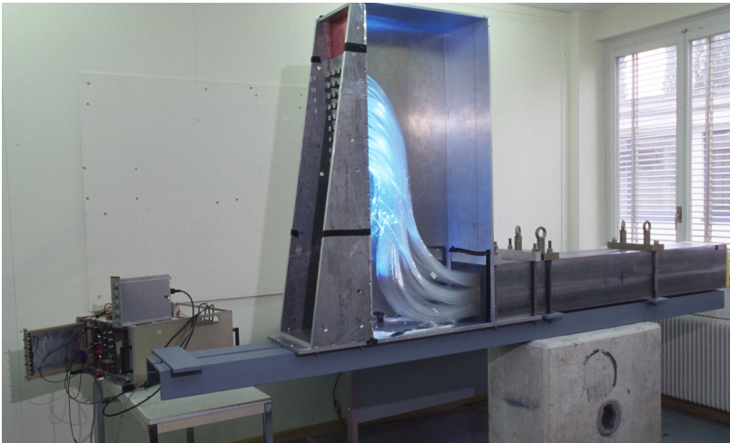
Figure 2.9: Photo of an HF tower before installation into CMS showing the quartz fibers [18].
