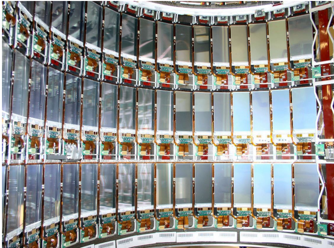
Figure 2.6: Photo of strip detectors in the tracker in the barrel region [16].
