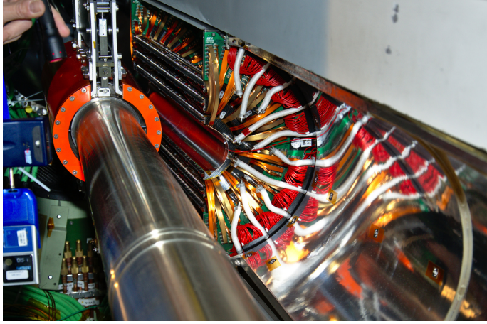
Figure 2.5: Photo of pixel detectors in the tracker next to the beam pipe [15].
