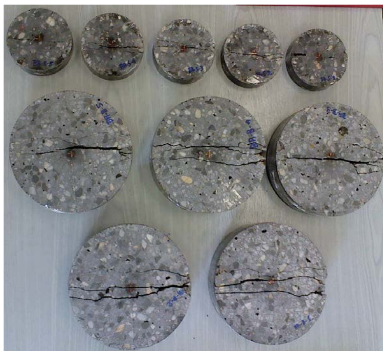
Figure 6-39: Epument samples after the Brazilian disc tests
