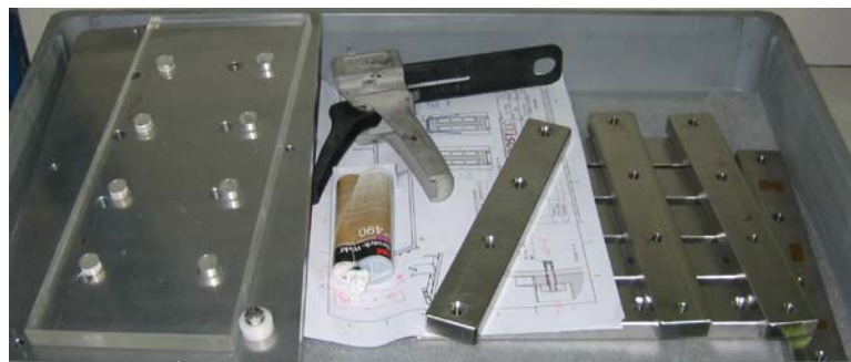
Figure 4-15: Girder metal plates for cradle fixation
