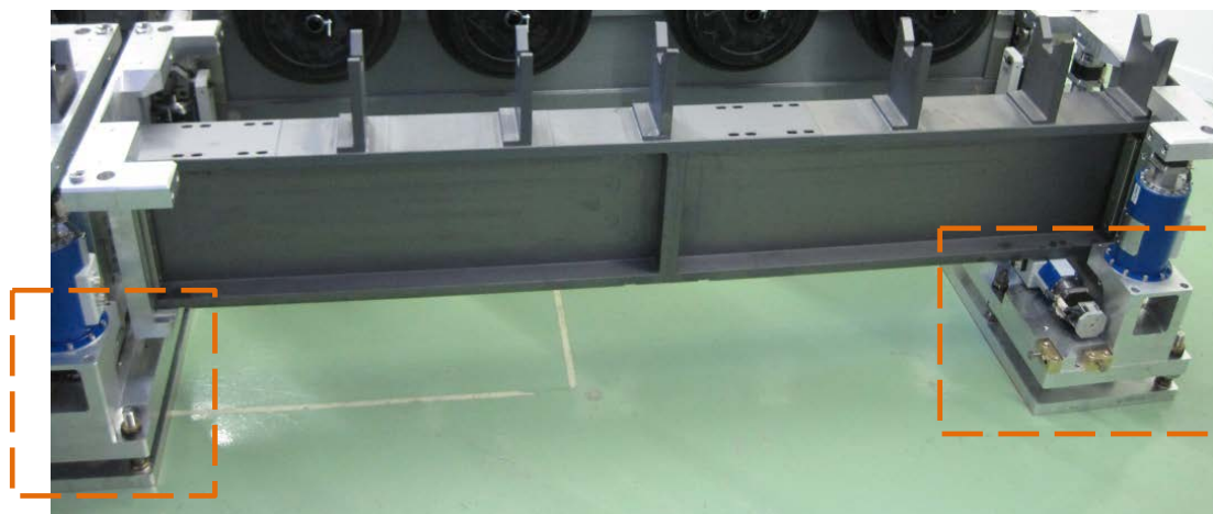
Figure 5-10: Alignment plates under the cradles creating rigid body modes
