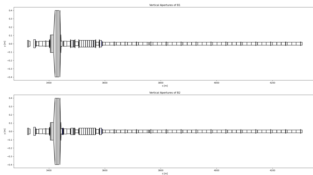
Figure 4.5: Vertical apertures and layout, IP2, the two beams are plotted separately. On the right side, we can see the beginning of the arcs
