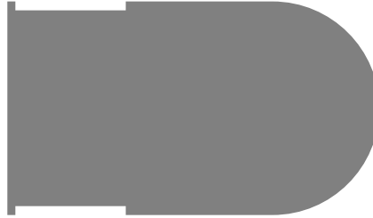
Figure 2.12: Aperture of the modules of the TDIS at parking position \pm 55mm . SVG path: M 0 4 h 78.4 a 60 60 0 0 1 0 120 h -78.4 h -4 v -5 h -62 v 5 h -4.5 v -120 h 4.5 v 5 h 62 v -5 z [7]
