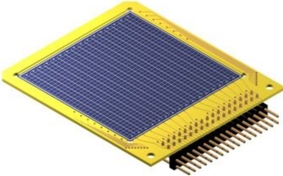
Figure 3.2: A schematic drawing of the DSSSD detector type. The detector has 16 vertical strips on the frontside, each of them separated by a so-called interstrip region. On the backside the detector has 16 horizontal strips also separated by interstrip regions. If a particle deposits energy in the interstrip region, it will not be detected by the detector. A strip is rectangular in shape and characterized by the fact that if a particle deposits energy in it, only this specific strip observes the signal. This is due to the fact that an electrical conductor is running along the strip. The combination of vertical and horizontal strips gives a position sensitive detector with 256 pixels in the case of a 16 \times 16 strip detector.
