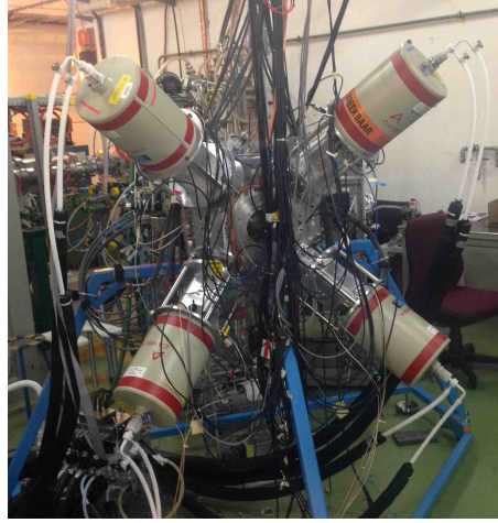
Figure 7.1: HPGe clover detector setup at the IDS. Collection chamber is at the central position where the four detectors meet.
