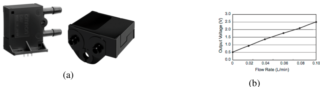
Fig. 2.1: (a)Photographs and (b) response of the flow-meter [3].
