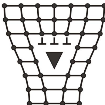
Figure 40 : Nucleation of a micro-crack due to accumulation of dislocations
