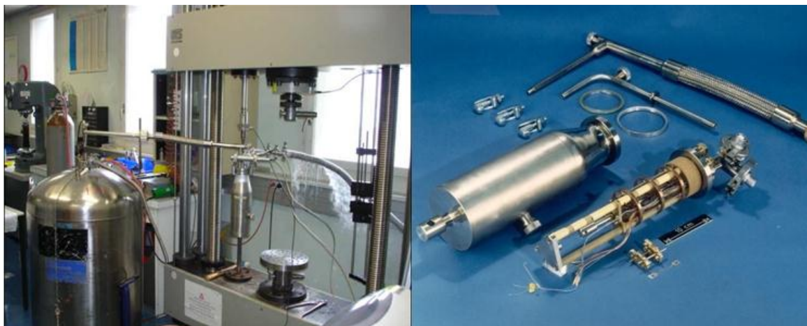
Figure 94 : The tensile/compression machine, cryostat and liquid helium
