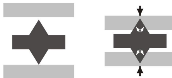
Figure 30 : Knife edges seal with hard gasket and soft flanges
