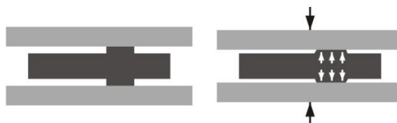
Figure 16 : Plane seals with gaskets of special shapes: gasket with beads
