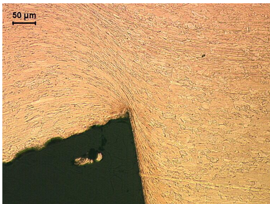
Figure 115 : The plastic flow near the knife tip
