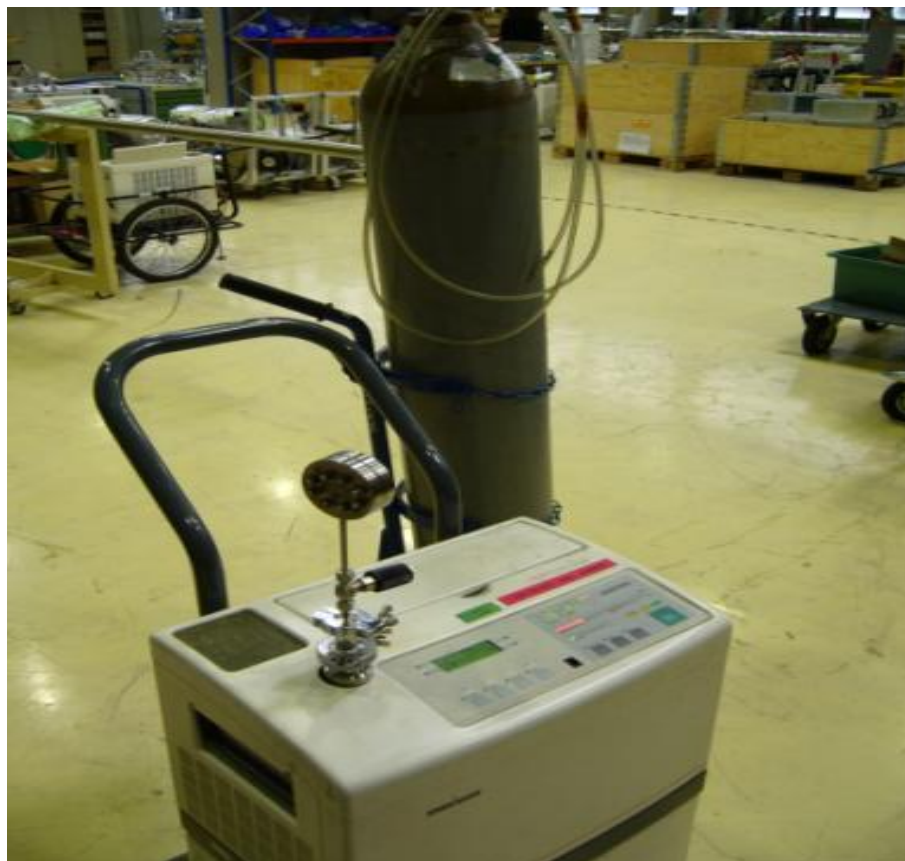
Figure 118 : Leak tightness testing setup
