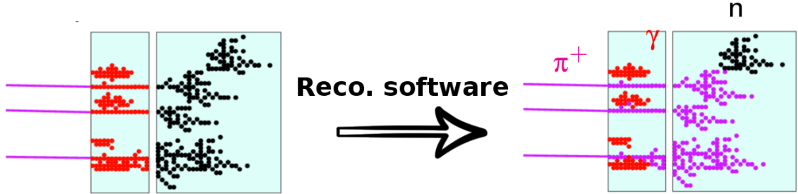
Figure 2.3: The separation of the jet components are made by the reconstruction software using the informations of the tracker and vertex detector and the highly granular calorimeters [9].
