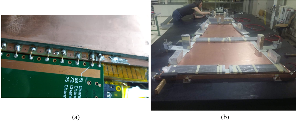
Figure 8.5: The ground connections are not performed for the pad channels on the quadruplets shown in (a). The support frame is glued on the first side of the wedge, as shown in (b).
