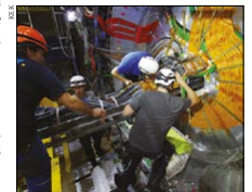
The vertex detector being incorporated into Belle II.
