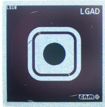
Fig. 7.: Photograph of n-LGAD sample produced by IBM-CNM studied in this work (top view of a device). The corresponding PiN sensors of the same producer look identical.
