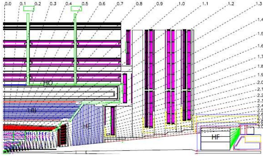
Figure 2.11. Cross section of the HCAL longitudinal view with the rest of the CMS.
