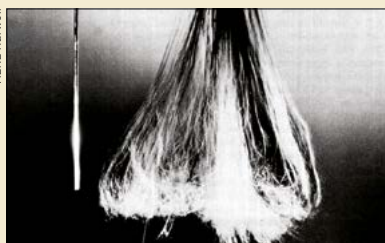
Nb_3Sn multi-filamentary conductors promise much higher fields and better temperature stability than NbTi. The wire on the left contains filaments that are revealed when the bronze matrix is etched away.
