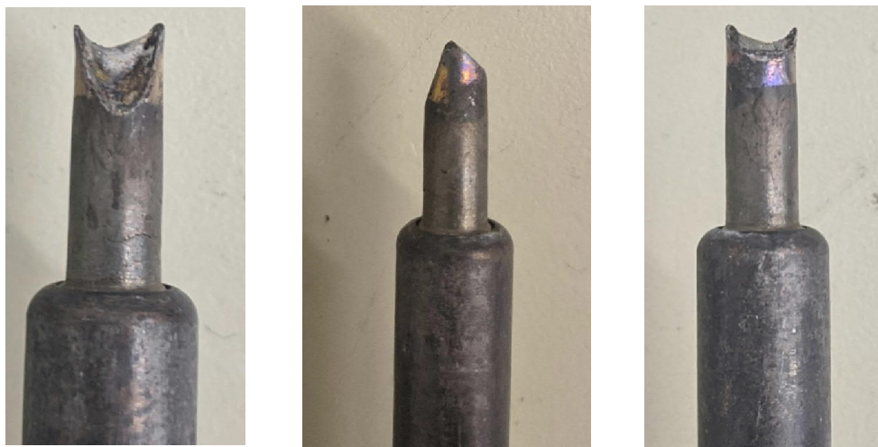
Figure 1 – Soldering iron with Kamil Cichy's custom shape.
