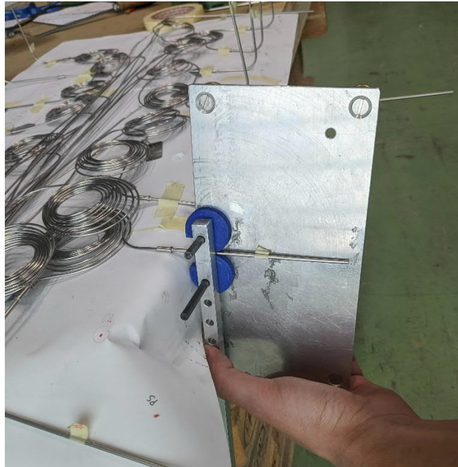
Figure 8 – Bending process in-situ.
