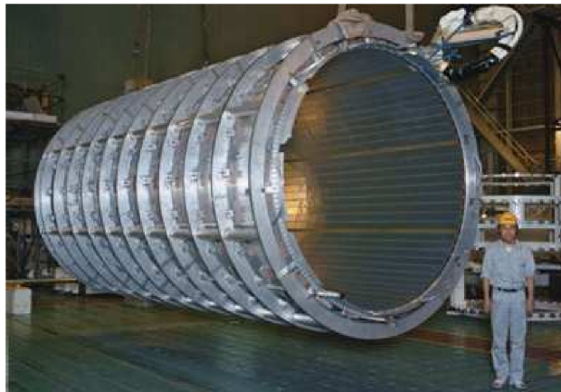
Figure 4.10: Bare central solenoid in the factory after completion of the coil winding [81].
