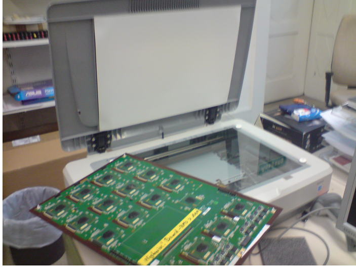
Figure 3.17: EPSON GT 200000 scanner used to take picture of the ROB for the identification of the MCMs.
